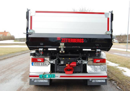
Spreader gate 40 mm aluminum profiles with front hinge 130 mm.
