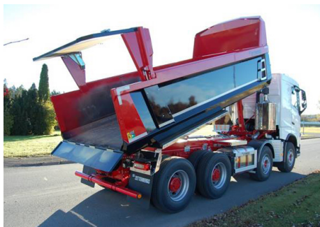
Spreader gate steel alt. aluminum high-lift incl. automatic tailgate. (Not for side tip.)
