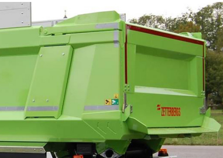
Spreader gate steel alt. aluminum high-lift with slide locking. Automatic tailgate is deleted. Bottom extended 200 mm. (Not for side tip.)
