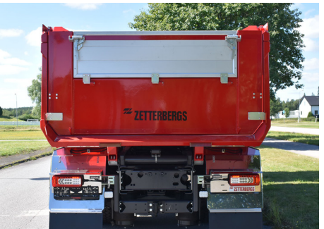
Spreader gate steel front-hinge with integrated and openable/removable aluminum hatch.
