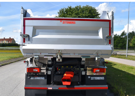
Spreader gate steel front hinge 250 mm. Top edge lowered 200 mm.
