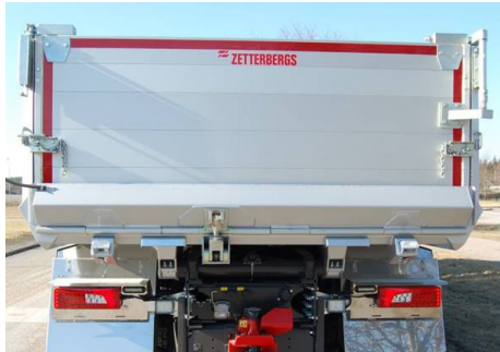
Spreader gate 40 mm alu-profiles, hanging and turning, door type.
