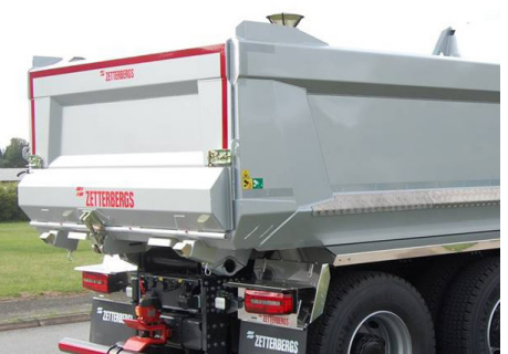
Spreader gate steel 5 mm with front hinge 130 alt. 250 mm.
